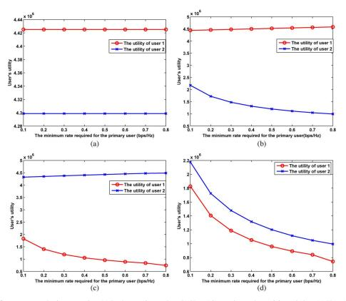
Fig. 5. User utility in four spectrum sharing scenarios. (a) Both users in overlay. (b) User 1 in overlay and user 2 in underlay. (c) User 1 in underlay and user 2 in overlay. (d) Both users in underlay.
